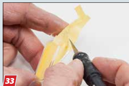
33 The sharply molded canopy's straight lines make masking the clear part easy. I applied Tamiya tape and burnished it into the frames, then carefully trimmed around them with a new, sharp No. 11 blade.
