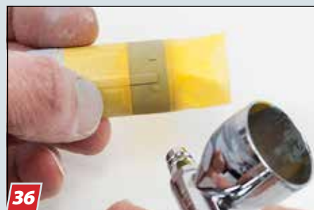
36 Most of the ribbed section on the engine sections on the S-foils were painted dark ghost gray, but I sprayed the front of the upper port section with a mix of equal parts insignia yellow and gull gray.
